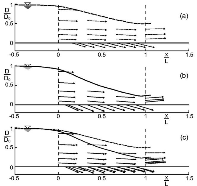
**Fig. 4.** Distribution of the velocity vector in a vertical plane passing through the axis of the slit between two adjacent bars, measured during (a) Run 2 ( $F_{r0}=2.05$ ,  $D_0=8$  cm) and (b) Run 8 ( $F_{r0}=1.20$ ,  $D_0=8$  cm); (c) comparison between the two velocity patterns: Run 2, thick line and Run 8, thin line
