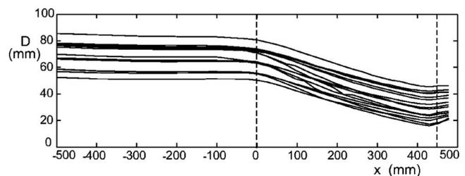
Fig. 2. Water depth profiles measured along the axis of the flume for all the experiments listed in Table 2; vertical lines denote the beginning and end of the bottom rack
