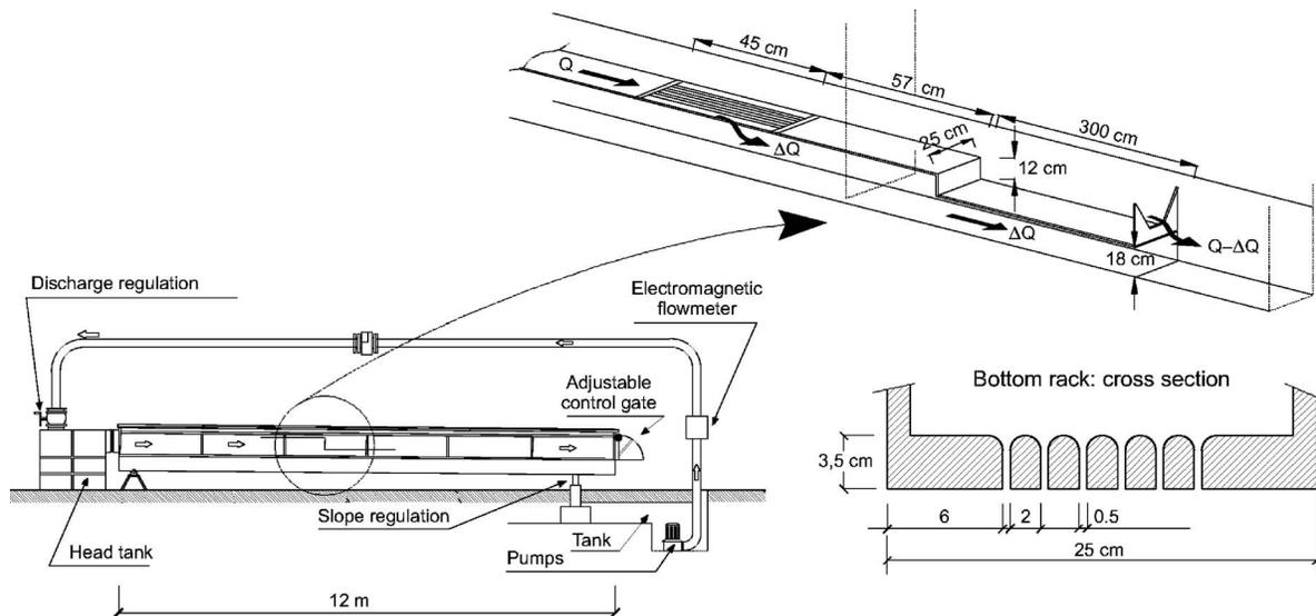
Fig. 1. Sketch of the experimental apparatus and geometrical characteristics of the adopted rack
