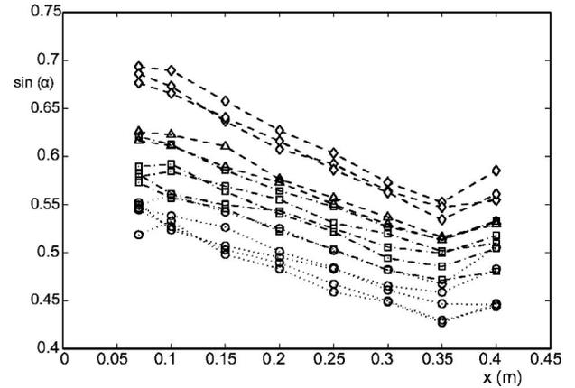
Fig. 7. Distribution of  $\sin \alpha$  in the slit between two adjacent bars 0.03 m below the bottom of the flume for all the experiments listed in Table 2. (○) Runs with  $F_{r0}$  in the range of 1.30–1.47; (△), runs with  $F_{r0}$  in the range of 1.70–1.82; (□) runs with  $F_{r0}$  in the range of 1.98–2.04; and (◊) runs with  $F_{r0}$  in the range of 2.21–2.33.
