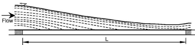
**Fig. 3.** Typical example of average streamlines observed in Run 10, reconstructed through PTV technique
